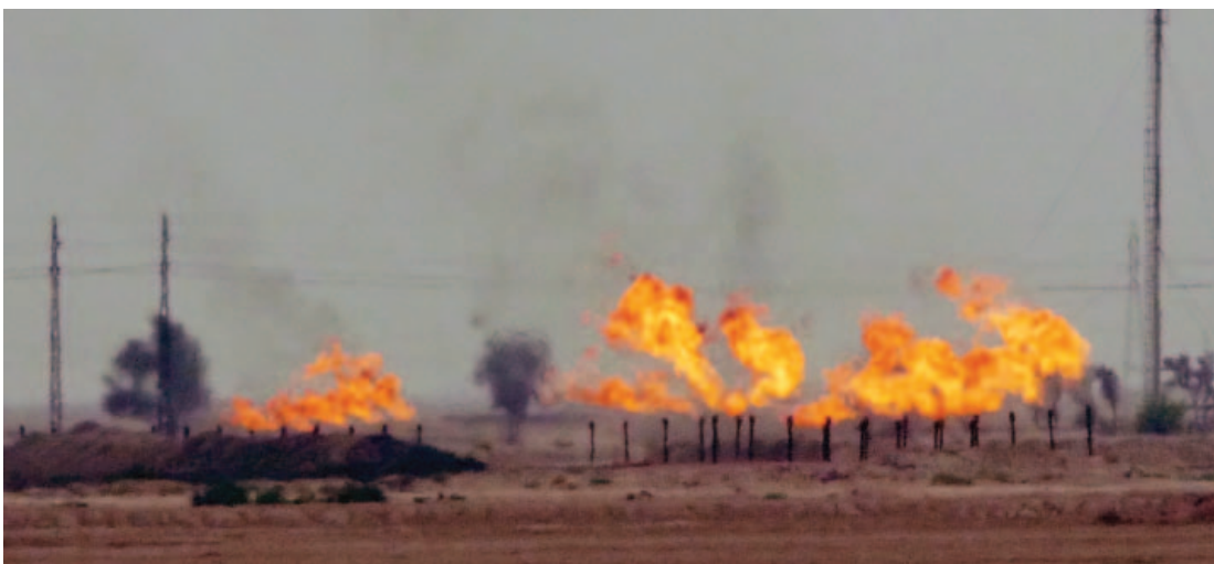
Gas flares in Rumaila oil field should be lessened by efforts currently under way by a Shell-led joint venture to capture associated gas from Rumaila, Zubair, West Qurna Phase One and Majnoon oil fields.
